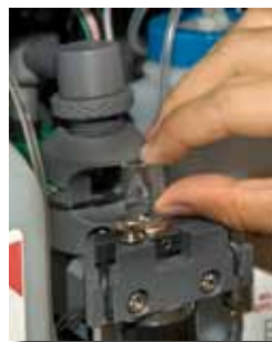
Changing the Sample Cuvette
