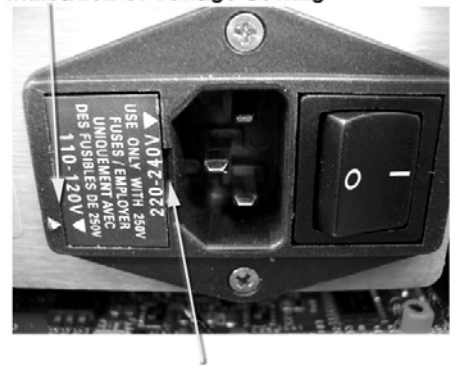
Insert a flat blade screwdriver to remove fuse cartridge
