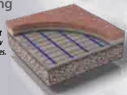
Concrete Slab: ProMelt mat or cable zip-tied to mesh or grid in the middle of the slab.
