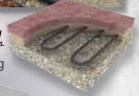
Slab on Grade: Radiant PEX+ tied to mesh or grid.
